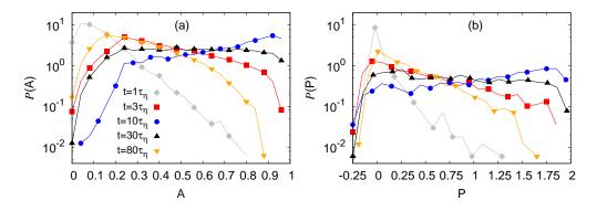
Figure 4: Probability density functions for the asphericity (a) and the prolateness (b), at various times,  $t = 1\tau_{\eta}(\diamondsuit)$ ,  $t = 3\tau_{\eta}(\Box)$ ,  $t = 10\tau_{\eta}(\bigcirc)$ ,  $t = 80\tau_{\eta}(\bigtriangledown)$ . Even at large times there is still a considerable number of puffs far from having a spherical shape.
