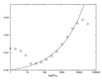
FIG. 2. Experimental  $F_{1,2}(r,R)$  at fixed  $r=16r_d$  and at varying R. The integral scale  $L\sim 1\times 10^4r_d$ . Let us remark that the observed change of sign in the correlation implies the presence of at least two power laws. The continuous line is the fit in the region r< R< L obtained by using only the first two terms in (10).
