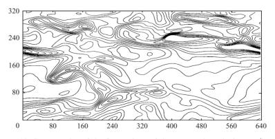
FIGURE 13. Contour plot of the fluctuations of the streamwise velocity at  $y^+ = 37$ .
