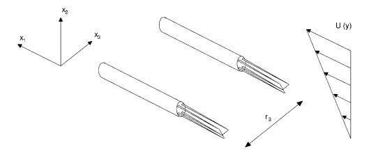
FIG. 3. Schematic of the measurement configuration: Each of the two X wires, separated in the transverse direction,  $z=x_3$ , detects two velocity components u and v (in the streamwise,  $x=x_1$ , and in the shear direction  $y=x_2$ , respectively). The separation between the two probes was measured by means of a charge-coupled device (CCD) camera with a high magnification lens and could be changed by means of a precision transverse gear from 0.8 mm to 70 mm.
