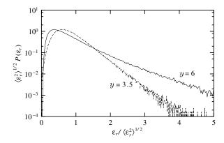
FIG. 4. PDF of the coarse-grained energy dissipation  $\mathcal{P}(\varepsilon_r)$ , for both y = 3.5 and y = 6.0, at the scale  $r = 8\eta$ .
