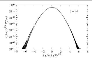
FIG. 3. PDF of the velocity increments, for y = 3.5. Scales are the same as the previous figure:  $r_1 = 34\eta$ ,  $r_2 = 74\eta$ , and  $r_3 = 114\eta$ .
